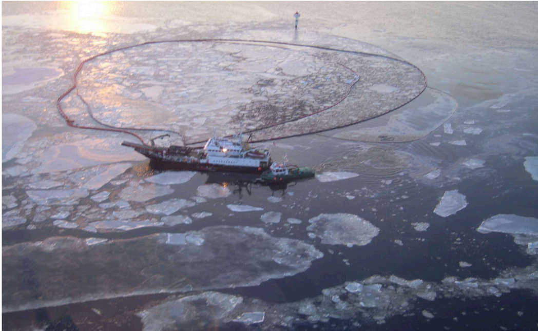
Figure 6: Godafoss Oil Spill (Norway, 2011) with a Double Boom Deployed in Ice-covered Waters.
