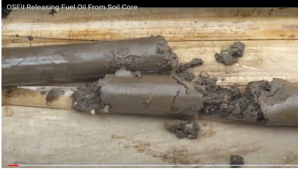
Soil Core sample contaminated with oil
